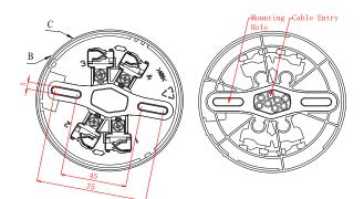
Warning: Do not punch mounting holes and cable entry holes bigger than needed. Do not punch more holes than needed.
