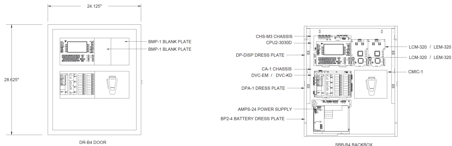
Figure 4.1.1 NFS2-3030 Configuration in SBB-B4 Backbox w/ Voice (Four SLC Loops)
